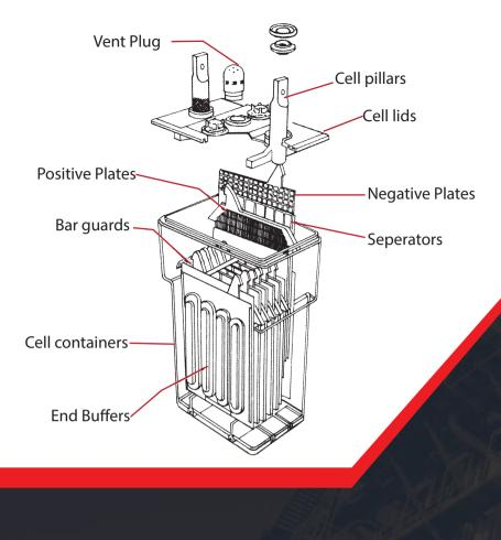
**Vent Plugs** - Specially designed incorporating a microporous ceramic filter which effectively returns all acid spray to all the cell, but allows free exit of oxygen and hydrogen which is generated towards the end of boost charging.
